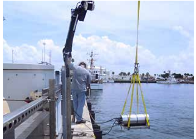
MIMS device being deployed over the sea wall in Bayboro Harbor at the SRI St. Petersburg facility.
