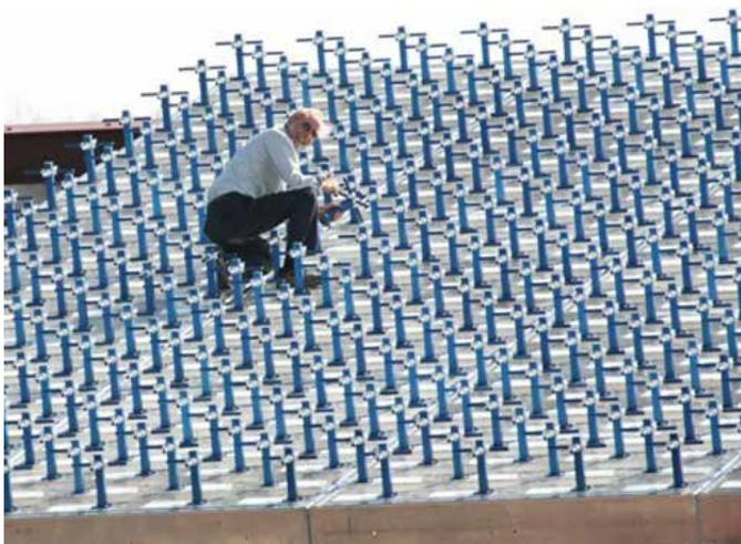
The novel modular configuration of AMISR allows relative ease of relocation for studying upper atmospheric activity around the globe. Remote operation and electronic beam steering allow researchers to operate and position the
