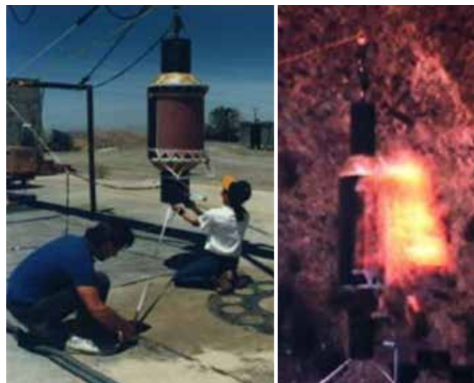
Figure 1. Impulsive loading with sheet explosive on a Kevlar/epoxy bottle to simulate X-ray loading.
