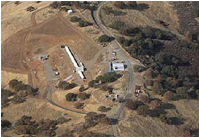
Figure 6. Aerial view of the 259-foot-long shock tube at CHES.
