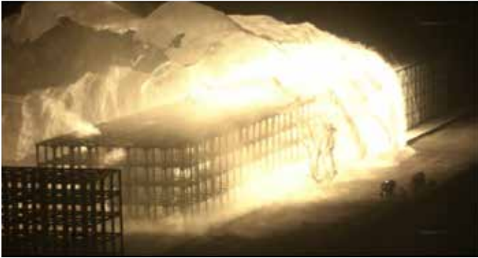
Figure 5. Large-scale flammable-gas deflagration to detonation transition.
