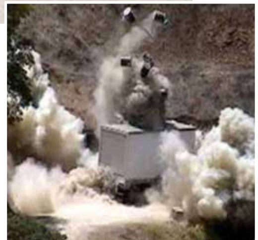
Figure 2. Neutralization of a vehicle bomb IED using SRI's DET.
